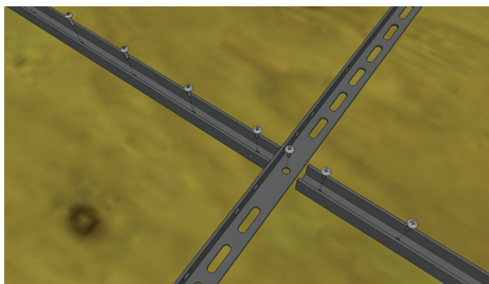
Figure F.2 - #10 x 3/4" flanged Phillips screws shown attaching to Aluminum Reinforcement Channels. Note that one is also placed through the center hole of the Interior Joist.
